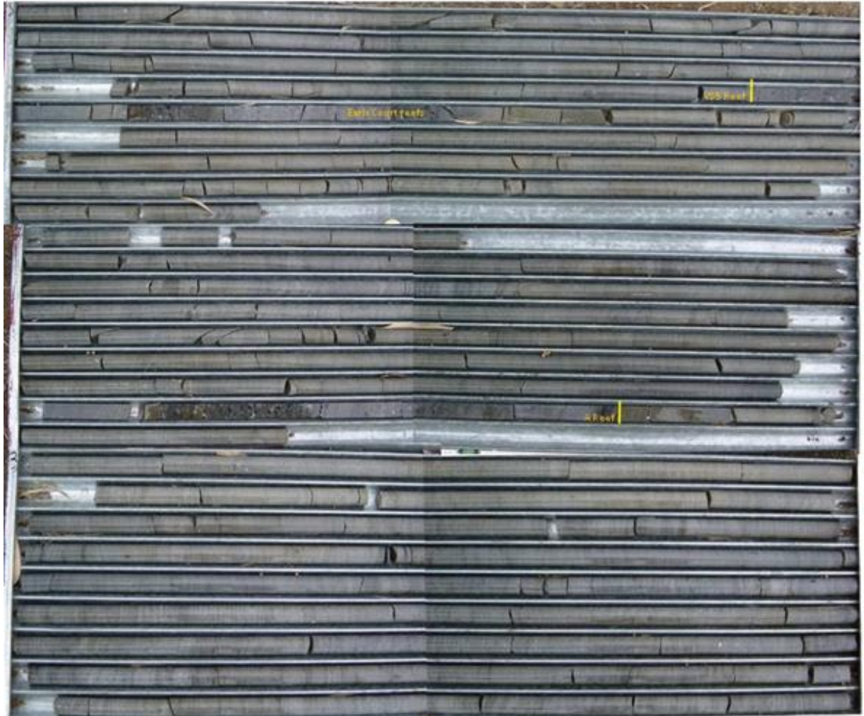
Plate 1: Photo-composite of upper part of the Kimberley Formation core from borehole HB1 mother hole
