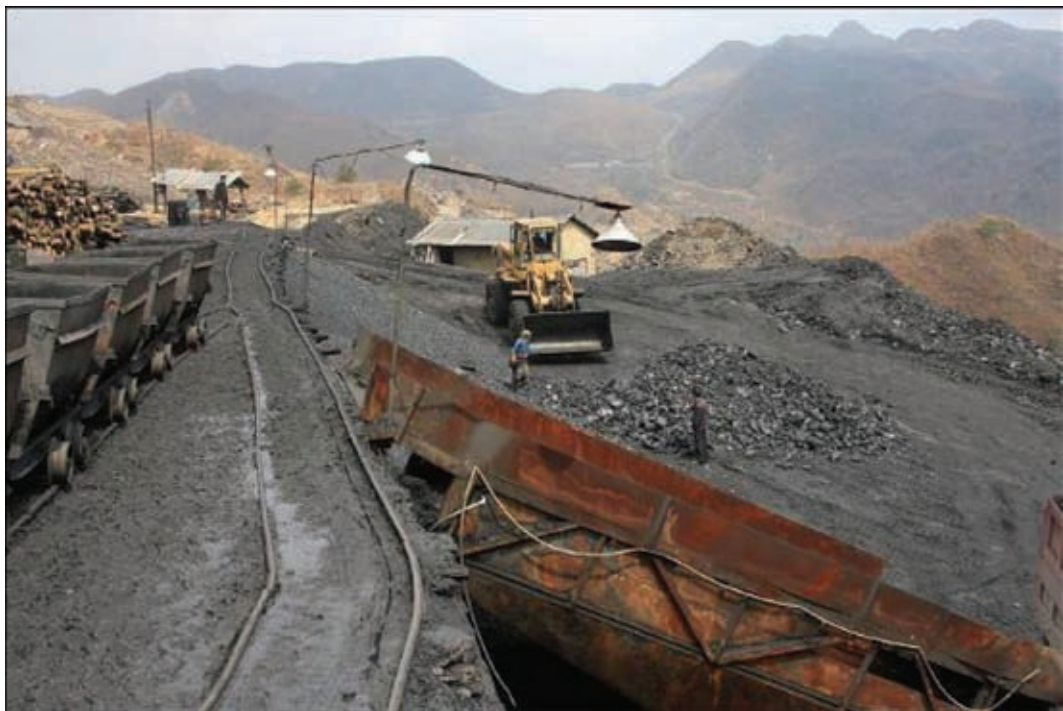
Figure 4 6: Stockpiling of Early Carboniferous Coal at the Xinghe Mine
